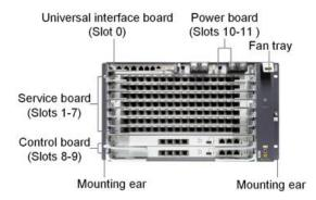
W x D x H Excluding mounting brackets: 442 mm x 268.7 mm x 263.9 mm Including IEC mounting brackets: 482.6 mm x 268.7 mm x 263.9 mm Including ETSI mounting brackets:
